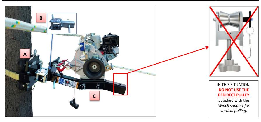
**ATTENTION** WHEN USED IN DIRECT LINE, THE PIVOTING ANCHOR FOR VERTICAL PULL SUPPORT (PCA-1332) MUST BE FIXED TO THE WINCH SUPPORT FOR VERTICAL PULL (PCA-2264). THIS ANCHOR (SOLD SEPARATELY) WILL ALLOW THE WINCH TO ALIGN WITH THE LOAD.
