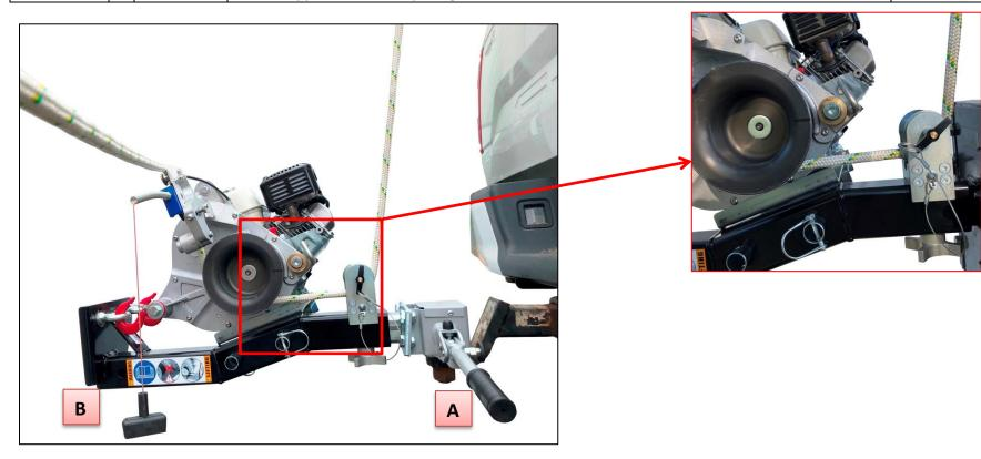
ATTENTION DO NOT GO OVER THE ROPE ENTRY PULLEY OF THE WINCH WITH THE ROPE AS IT WILL CREATE FRICTION AND WILL REDUCE LIFTING CAPACITY. GO UNDER THE ROPE ENTRY PULLEY OF THE WINCH. IN THIS CASE, THE ROPE ENTRY PULLEY OF THE WINCH WILL NOT BE USED.
