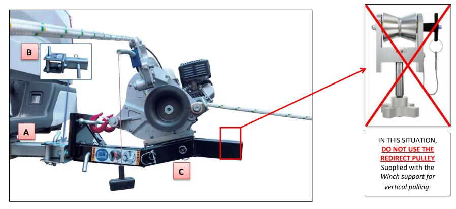
**ATTENTION** WHEN USED IN DIRECT LINE, THE PIVOTING ANCHOR FOR VERTICAL PULL SUPPORT (PCA-1332) MUST BE FIXED TO THE WINCH SUPPORT FOR VERTICAL PULL (PCA-2264). THIS ANCHOR (SOLD SEPARATELY) WILL ALLOW THE WINCH TO ALIGN WITH THE LOAD.
