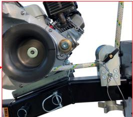
ATTENTION DO NOT GO OVER THE ROPE ENTRY PULLEY OF THE WINCH WITH THE ROPE AS IT WILL CREATE FRICTION AND WILL REDUCE LIFTING CAPACITY. GO UNDER THE ROPE ENTRY PULLEY OF THE WINCH. IN THIS CASE, THE ROPE ENTRY PULLEY OF THE WINCH WILL NOT BE USED.
