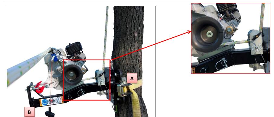
ATTENTION DO NOT GO OVER THE ROPE ENTRY PULLEY OF THE WINCH WITH THE ROPE AS IT WILL CREATE FRICTION AND WILL REDUCE LIFTING CAPACITY. GO UNDER THE ROPE ENTRY PULLEY OF THE WINCH. IN THIS CASE, THE ROPE ENTRY PULLEY OF THE WINCH WILL NOT BE USED.
